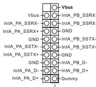
There is one header on this motherboard. This USB 3.1 Gen1 header can support two ports.
